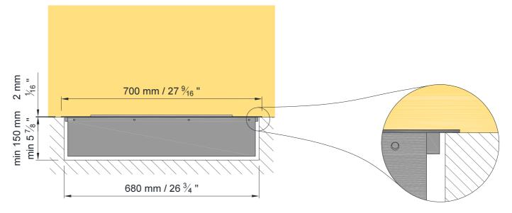
Make a cavity for the insert following the diagram below. Making the cavity make sure that the plane on which you are going to set the furnace inset is well levelled, as later it will not be possible to level the insert.
